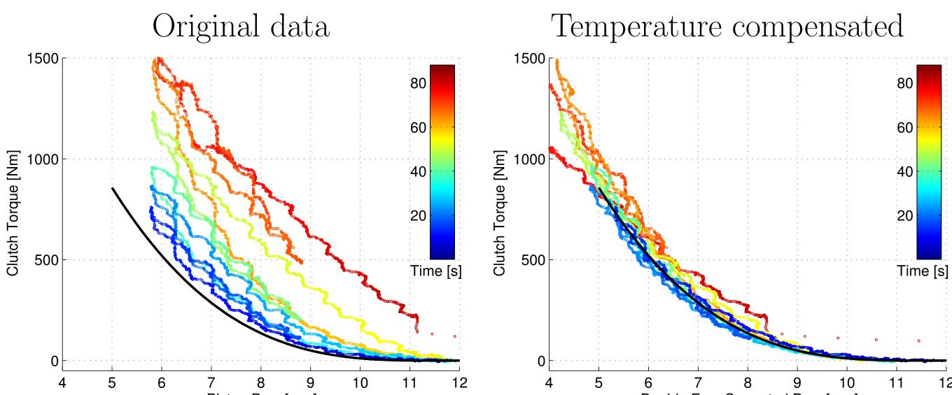
Double Exp. Corrected Pos. [mm] Left graph shows data of the torque drift when energy is dissipated into the clutch. Right graph shows the data after the position has been corrected for temperature effects using the clutch model developed in this project. The clutch model is a linear temperature model together with a linear thermal expansion.
