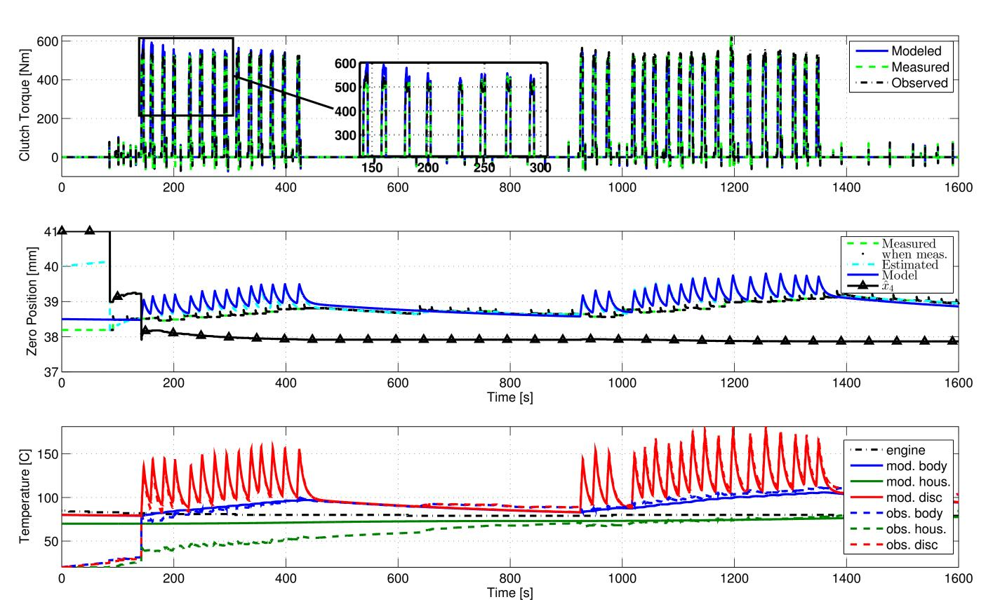
An Extended Kalman Filter has been built in order to handle unknown initial values and wear. The observer can start to converge before the clutch is being slipped by using the available measurement of  $x_0$ , see figure to the left.
