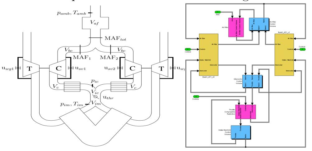
To model surge the compressor model must handle the reverse mass flow. This is achieved by the well known and well tested More-Greizer model.
