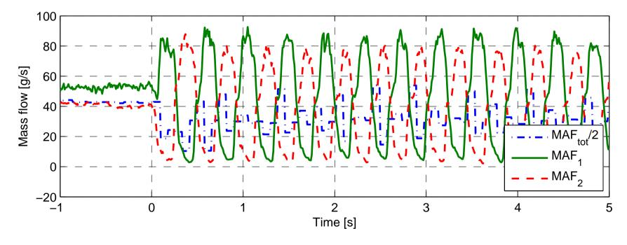
When the first compressor recovers it pushes the other into surge, starting an oscillation where the two mass flow alternately reverses.
